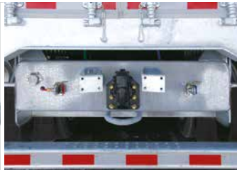
Pintle hook with air and electrical connections
