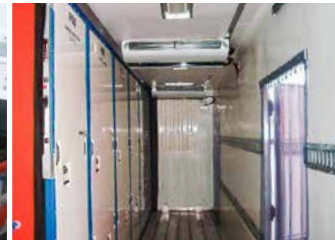
Various multi-temp configurations with remote evaporators available
