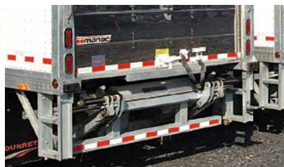
Door frame ready for installation of tailgate
