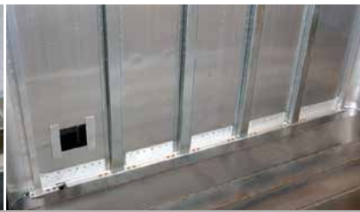
Heavy Duty six post front wall design Benefit: Increases strength
