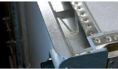
Outboard-mounted roof rivets Benefit: Impermeability and simplifies maintenance
