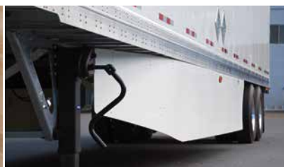
Aerodynamic skirt. SmartWay™ certified
