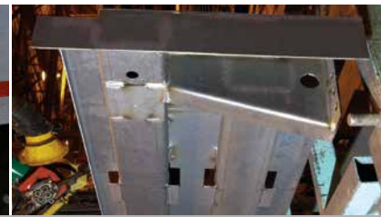
24" steel rear floor extension Benefit: Eliminates deterioration of wood floor at rear
