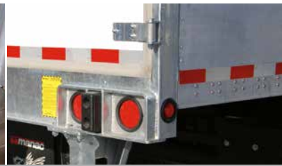
Rear connection with solid stainless steel rivets (32) Benefit: Superior bottom rail strength and reinforcement
