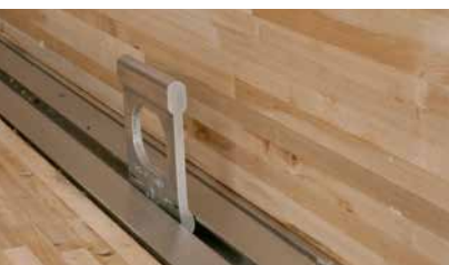
Floor-integrated securement track with multiposition cargo hands
