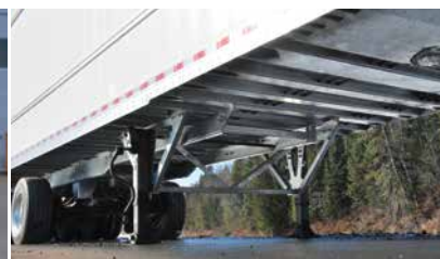
Galvanized steel coupler plate, crossmembers, tracks and bogie
